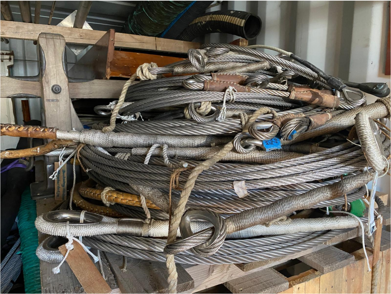
Figure 45 – Stainless steel standing rigging.
