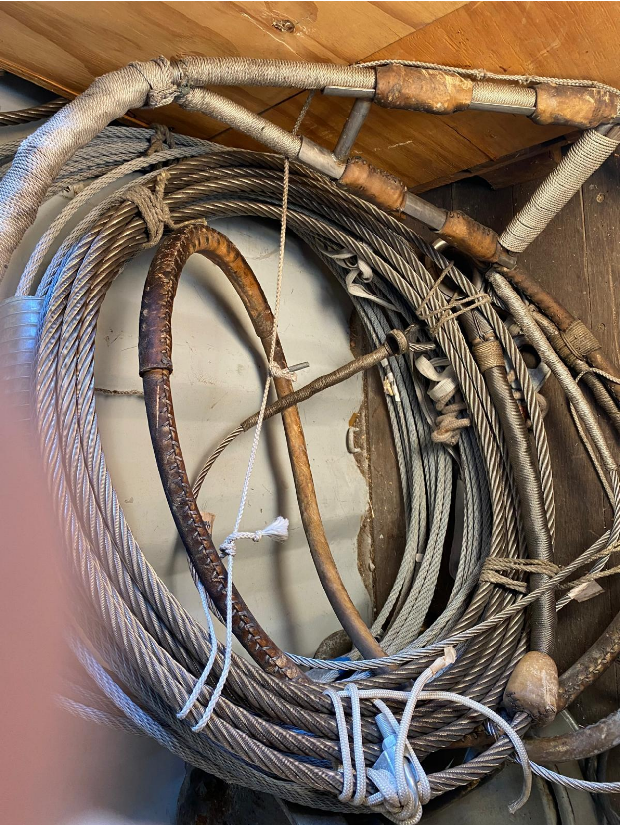
Figure 44 – Stainless steel rigging.
