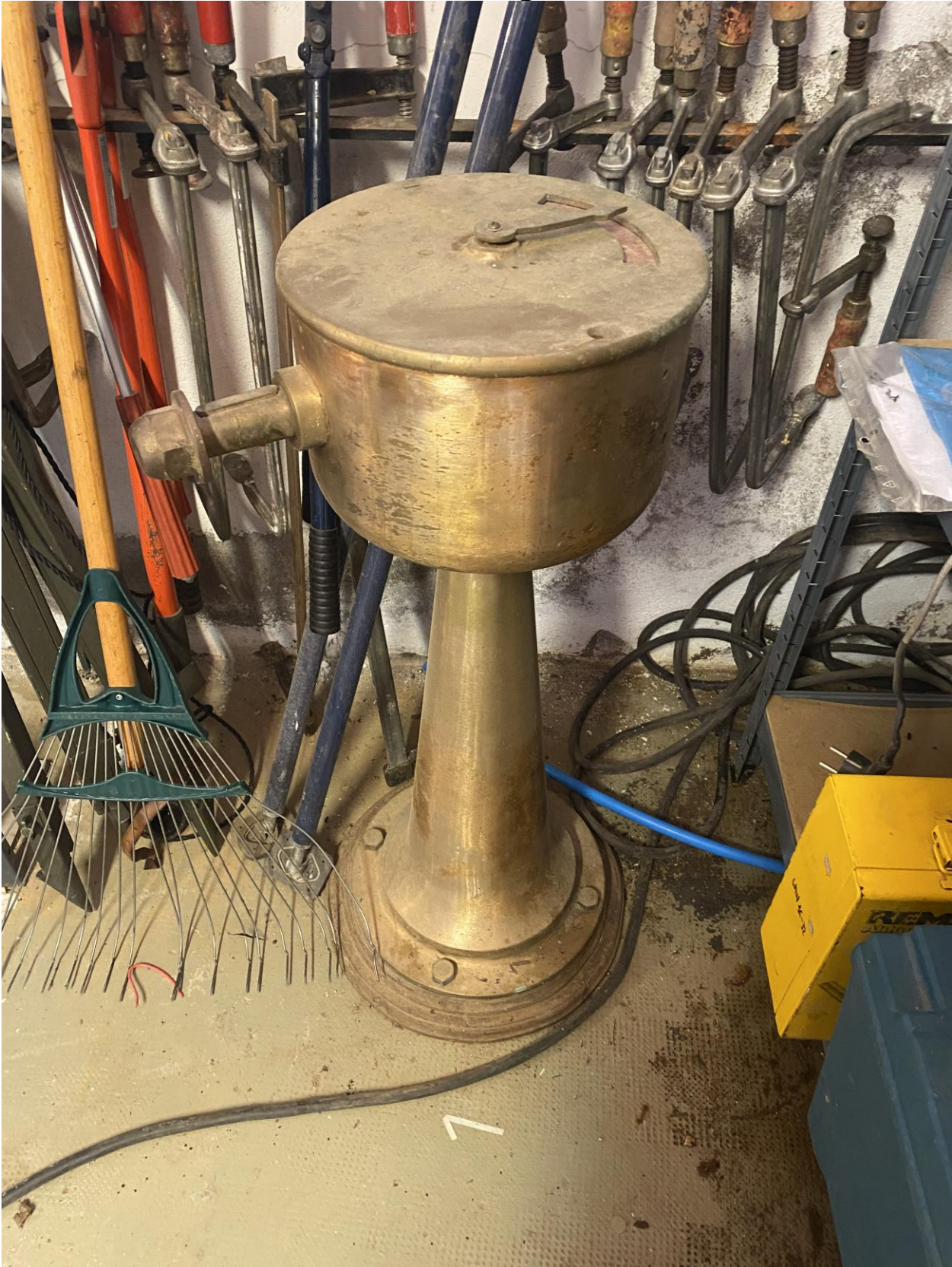
Figure 32 – Steering column with rudder angle indicator.
