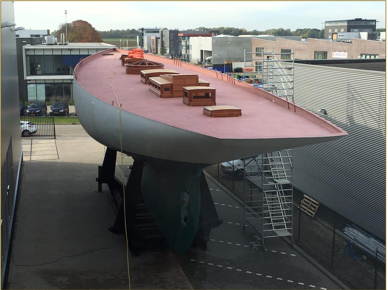
Figure 17 – Showing the deck with the deckhouses in place.
