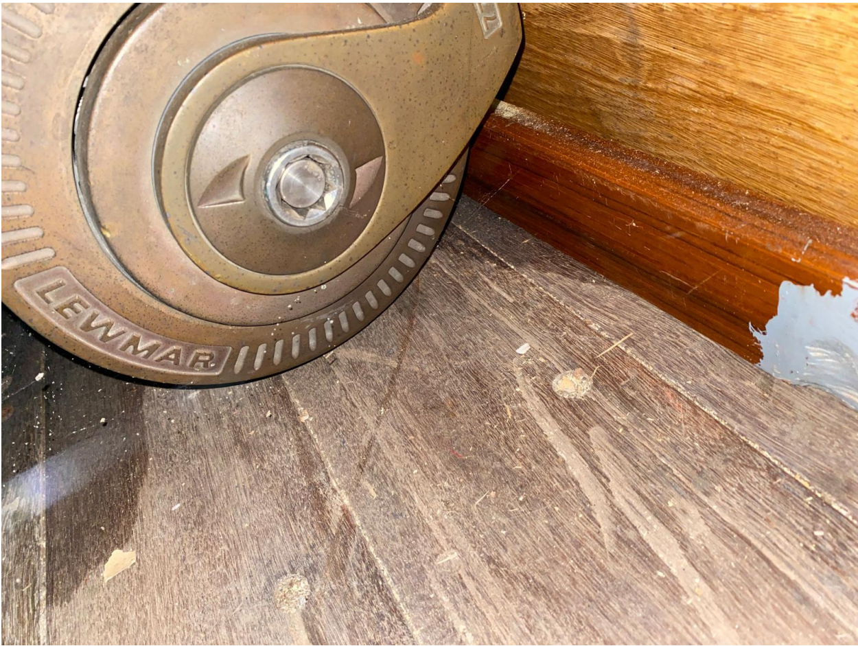
Figure 52 – Top of a Lewmar Bronze Hydraulic Winch
