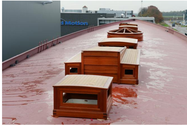
Figure 23 – Temporary alignment of deckhouses...
