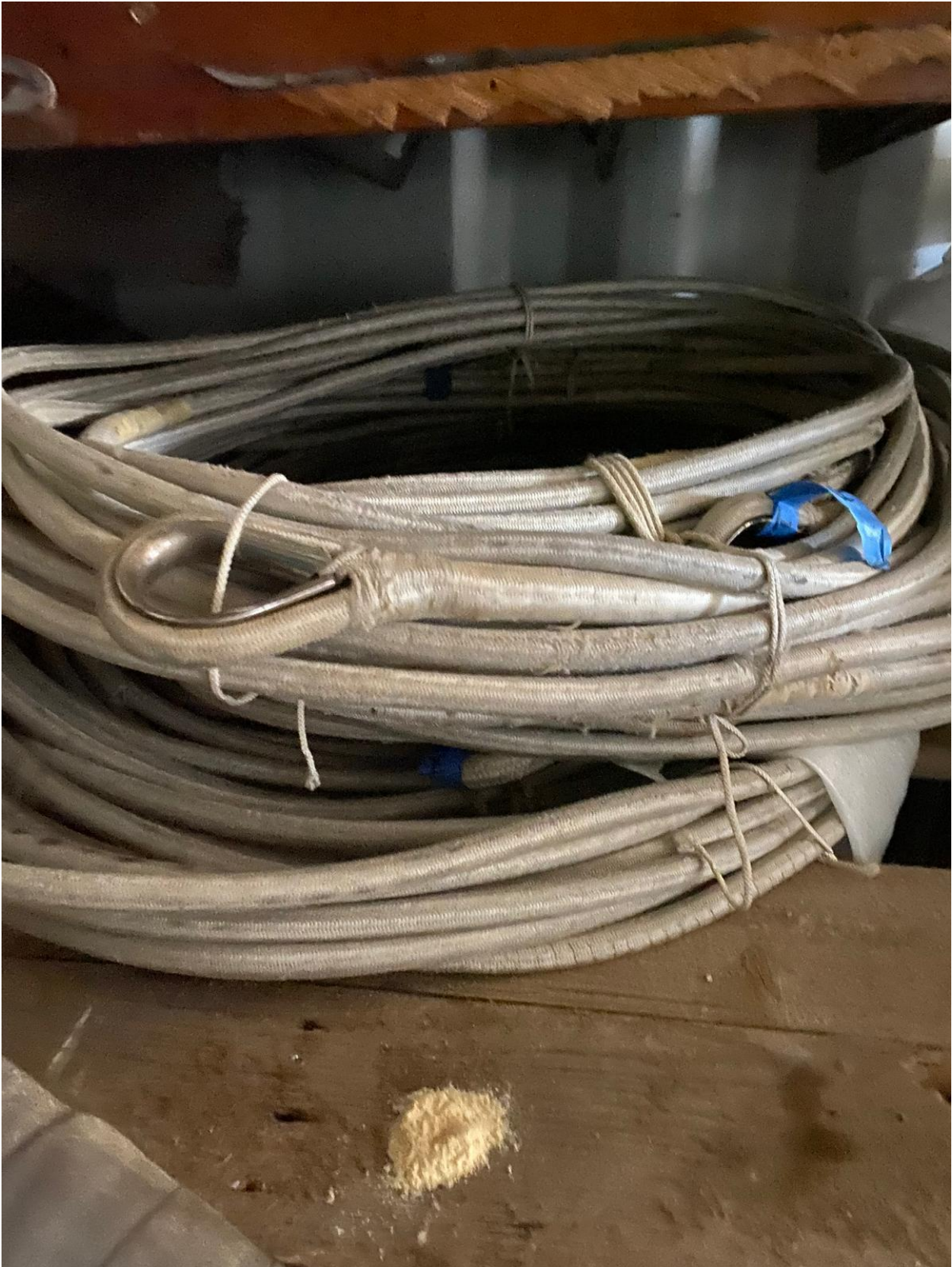
Figure 46 – Served standing rigging.
