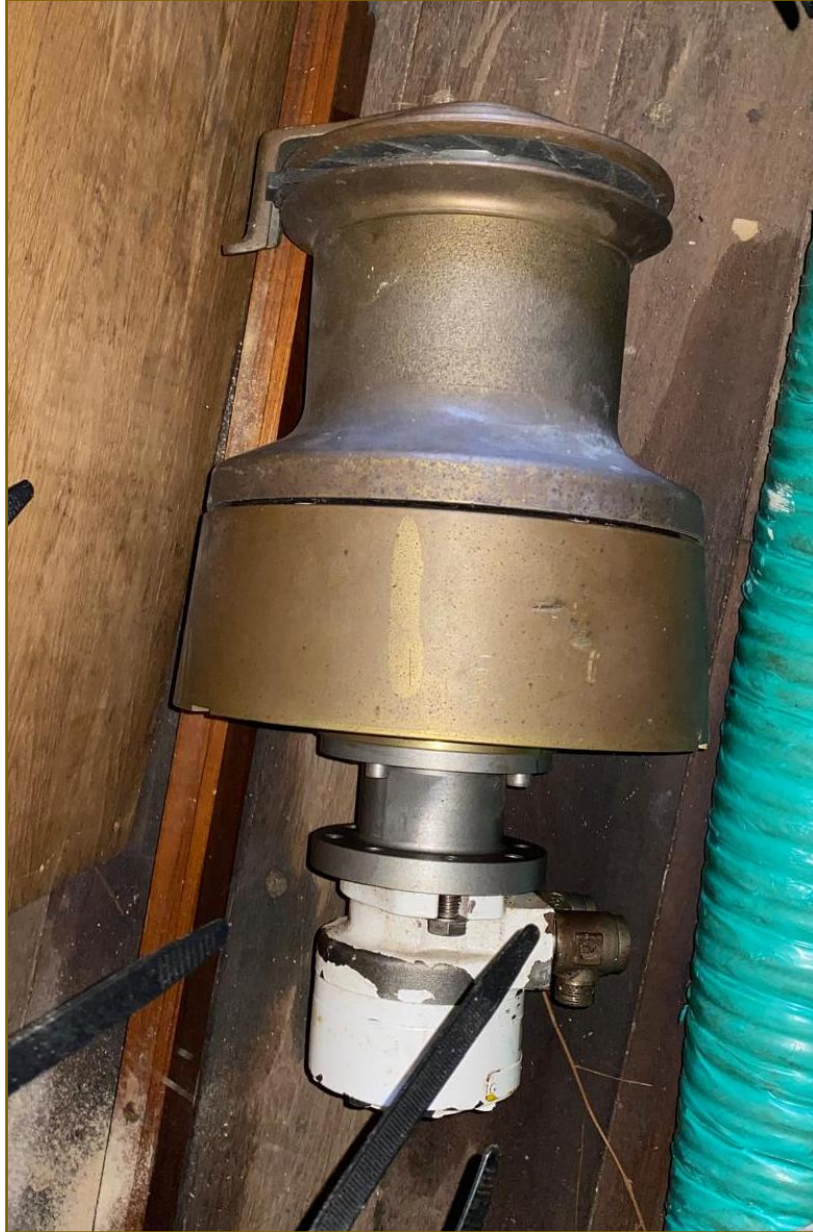
Figure 63– Lewmar Bronze Hydraulic Winch.
