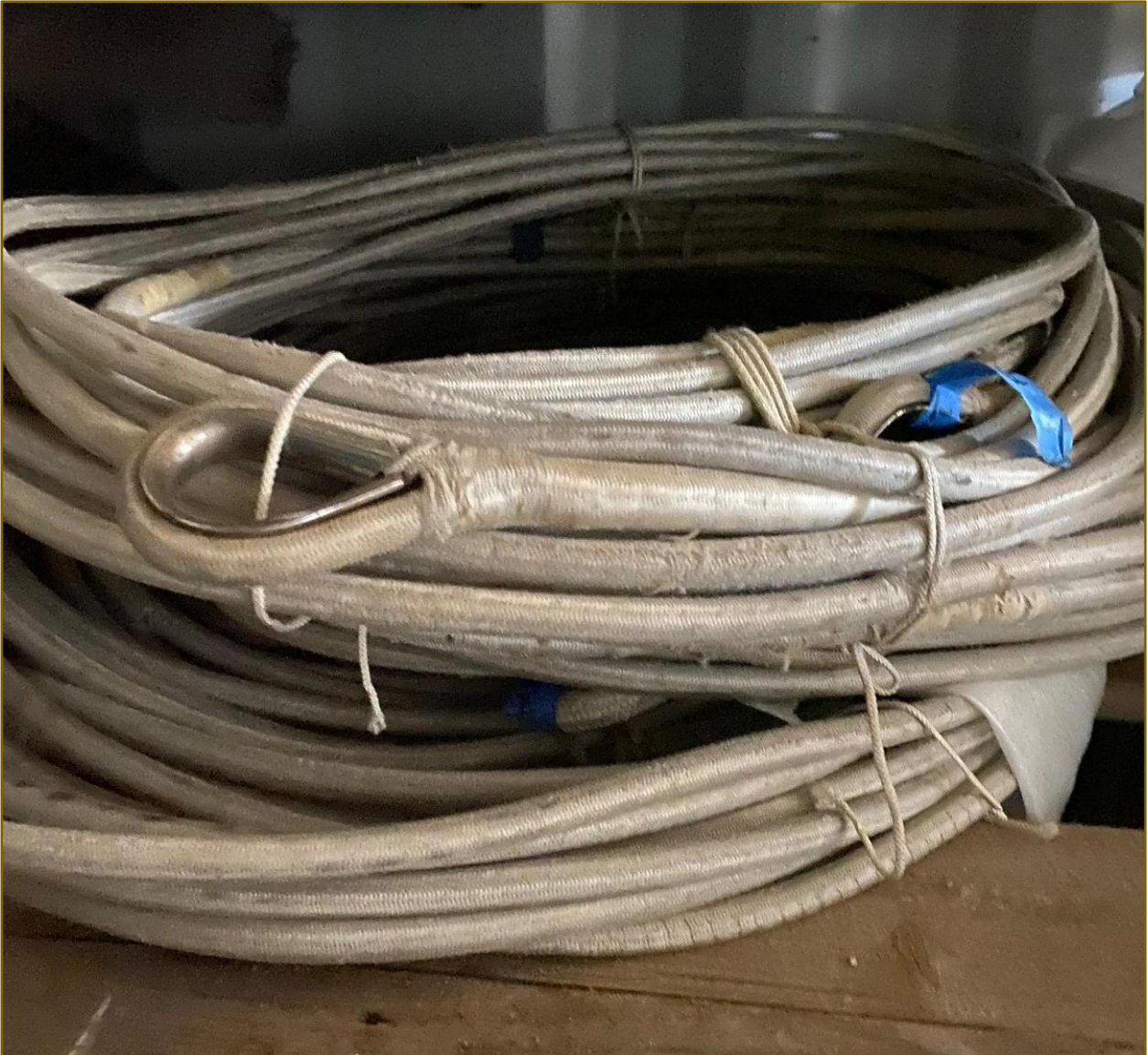
Figure 49 – Served standing rigging.
