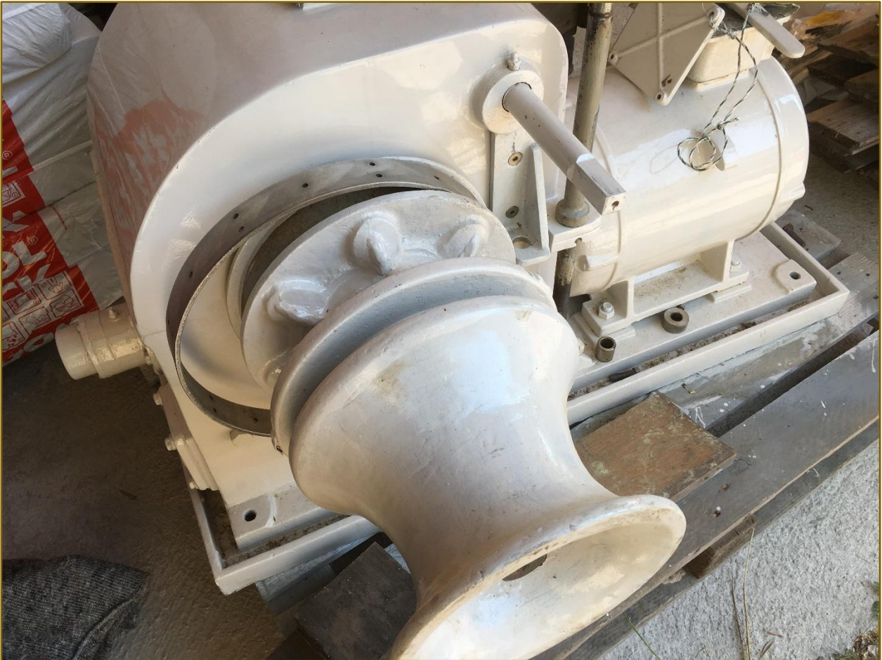
Figure 66 – Restored Thomas Reid Powered Windlass.
