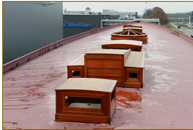
Figure 22 – Temporary alignment of deckhouses...
