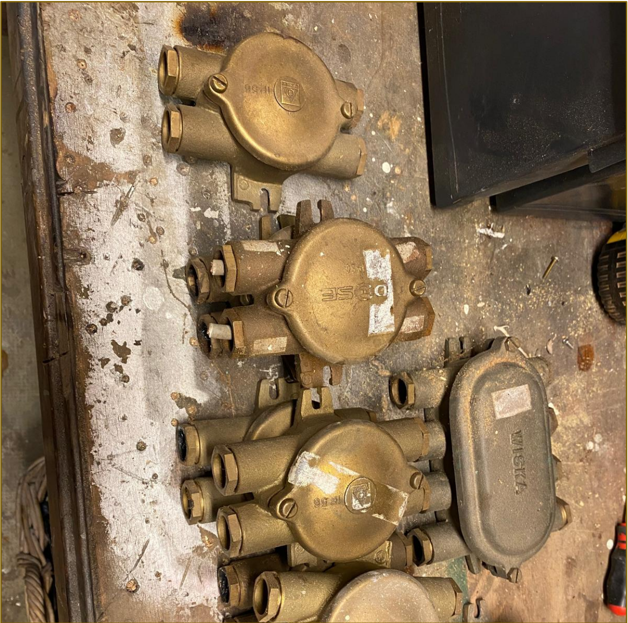
Figure 59 – More Wiska Bronze Water-Resistant Electrical Fittings
