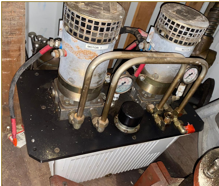
Figure 65 – Lewmar Twin Hydraulic Power Pack
