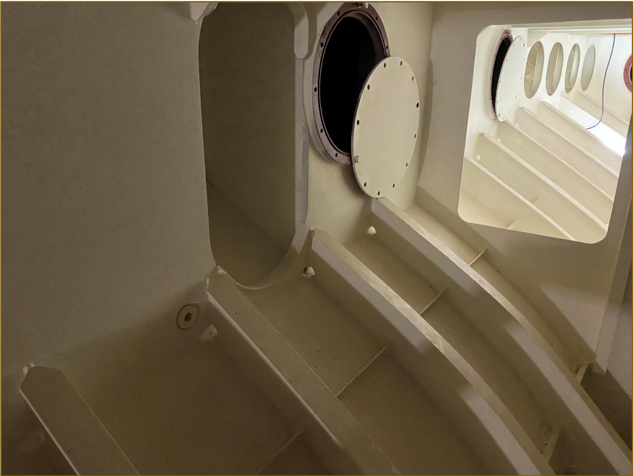
Figure 12 – The Engine Room showing frames, cofferdam and integrated tanks.
