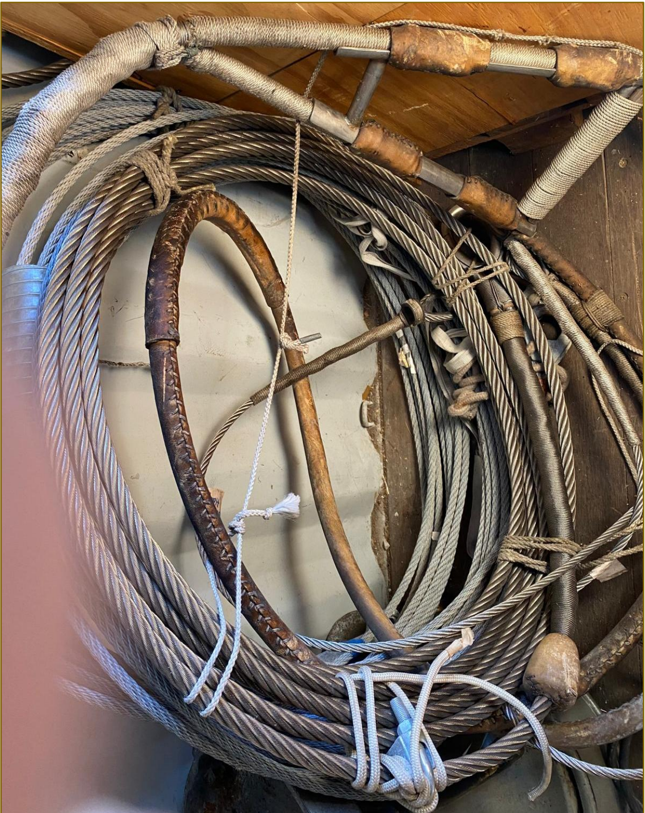
Figure 47 – Stainless steel rigging.
